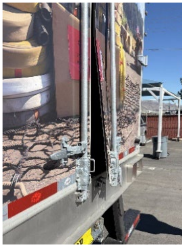
Three images depicting damage to the lower left corner of the right trailer door.
