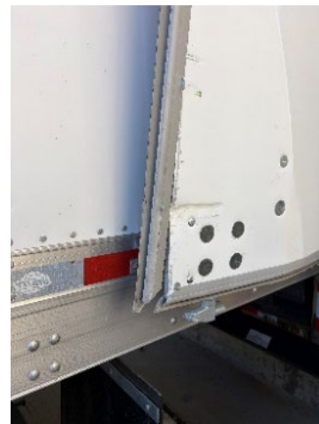
Three images depicting damage to the lower left corner of the right trailer door.
